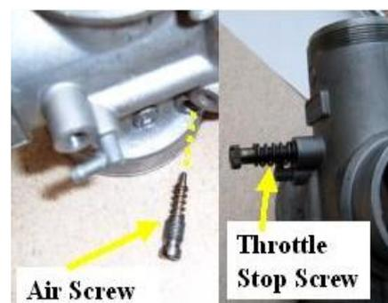
Replace the throttle stop screw, again gently turning fully in and then backing out ½ a turn.
