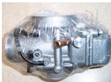
Now at this stage in an effort to maintain carb cleanliness and not undo this careful preparation, I always wrap my re-built carbs in cling film and then a soft clean rag to protect against knocks, only refitting to the engine on race day. This practice I find also helps to eliminate any condensation issues with warm carbs when stored in a cold garage. That said a good carb should always be kept warm under your pillow!
