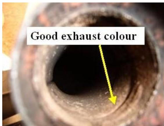
Come in, change to the next appropriate jet, record the air temperature and go out to test some more. You will quickly arrive, using this process, at the optimum main jet for the current conditions. When you do, record your setup and the air temperature for future reference. Another method used to check the main jet is to slowly lift the carb choke lever as you are driving down the straight, if the engine slows you are too rich if it picks up you are too lean.
